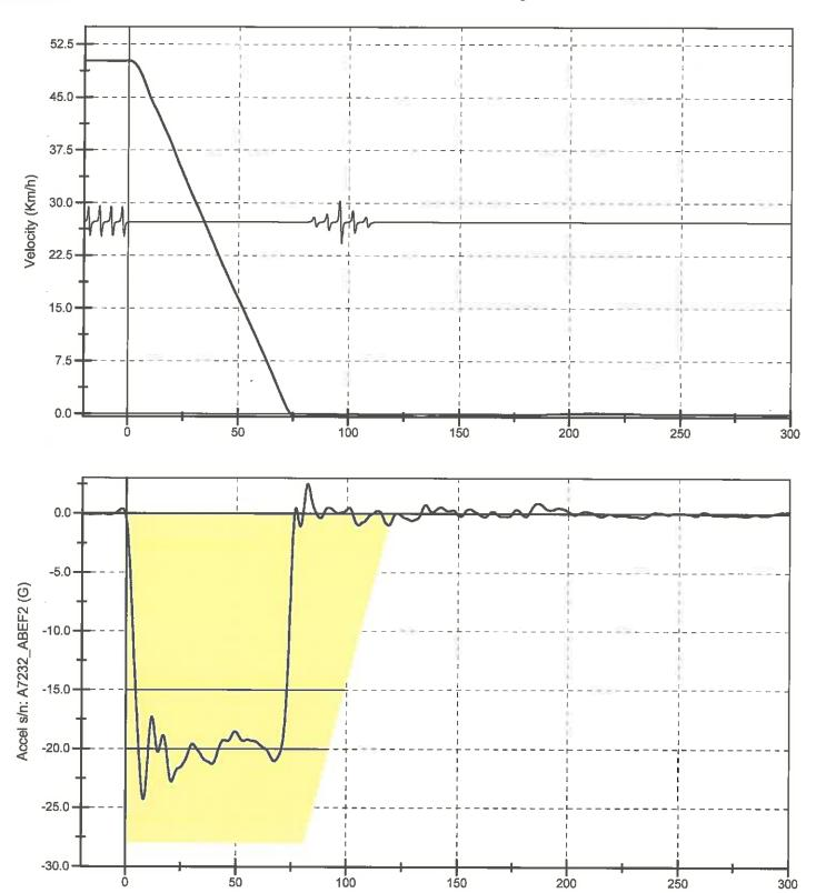
Continuous time under -15.0 G was 68.0 ms Total time under -20.0 G was 31.3 ms Sled Decel Peak = -24.3 G Sled Plateau Average Level = -20.4 G Sled Pulse Duration = 76.4 ms
